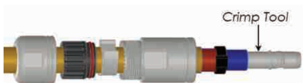
Step 5: Crimp terminal to conductor
