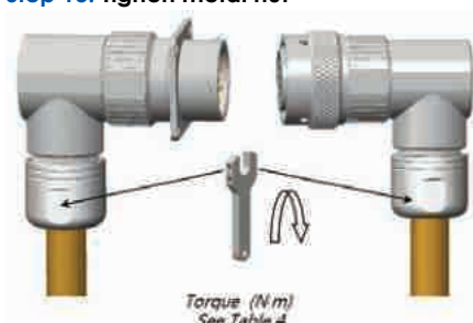
Step 13: Tighten metal nut
