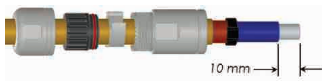
Step 6: Slide plug onto crimped terminal assembly
