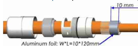
Step 4: Wrap foil over braided shielding
