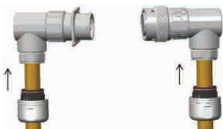
Step 11: Push shielding clip into backshell
