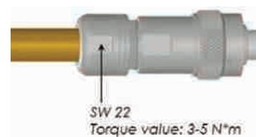
Step 8: Insert shielding clip and cable grommet. Attach and tighten back-nut to backshell
