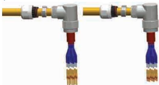
Step 7: Attach contacts to wire leads
