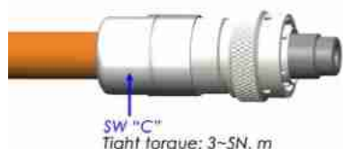
Step 9: Attach and tighten backshell as shown
