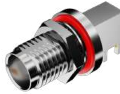
RFPC-TNC01-FN IP67/68 Right Angle DC to 4GHz Brass, Nickel Plated
