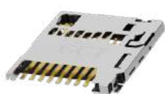
MEM2080 1.28mm Profile Push-Push 5000 Mating Cycles
