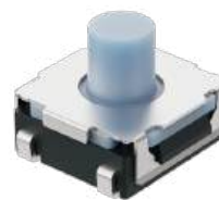
SWT7405 IP67 100,000 Life Cycles 400gf Actuation Force
