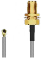
CAB468RF IPEX MHF I Plug to RP SMA Straight 1.13mm \varnothing Coaxial Cable DC to 6GHz
